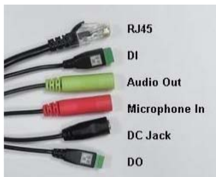
RJ45/ DI / Audio Out / Mic. In / DC Jack DO / Video Out (BNC)
